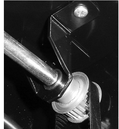
Top right idler screw and pulley
